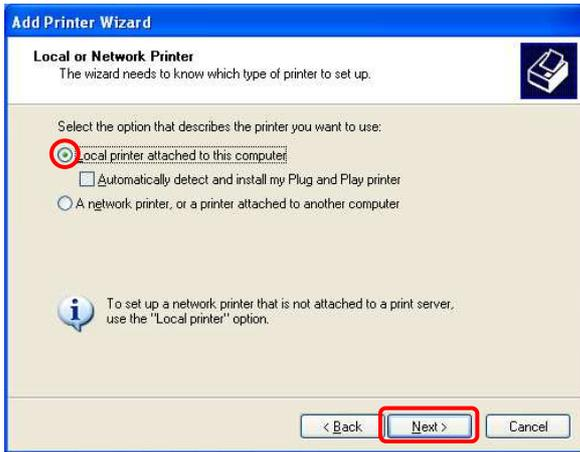
10. Select "Local printer attached to this computer" and uncheck "Automatically detect and install my Plug and Play printer", and then click "Next".
