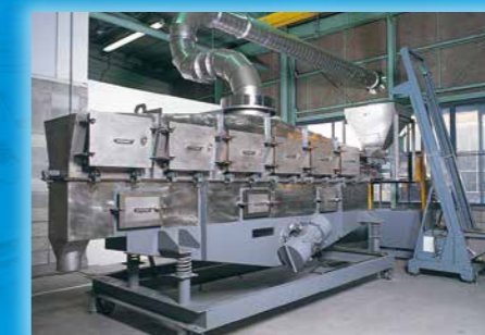
Test installation for vibrating drying and cooling processes
