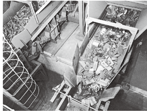
Feeding of melted material / scale and composite device (Hopper, vibrating conveyor, electromagnetic feeder)
