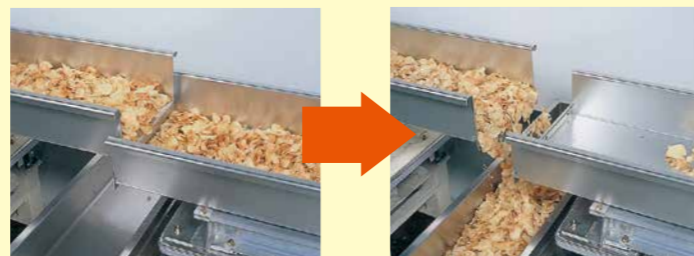
By moving the trough itself, it works same as a slide gate.
